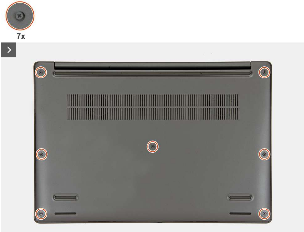
Figure 14. Loosen the captive screws
