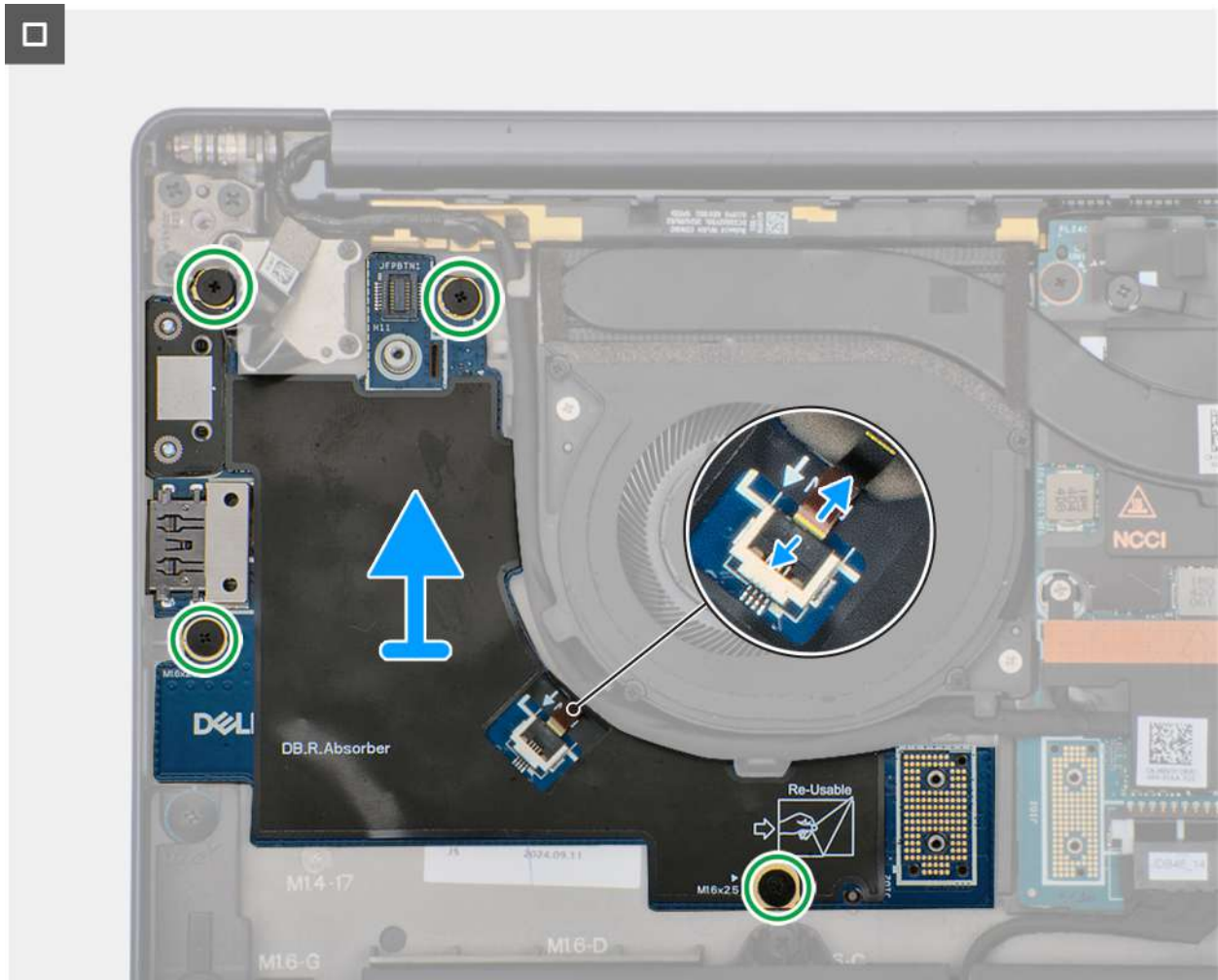
Figure 42. Removing the right I/O-board (without WWAN antennas)
