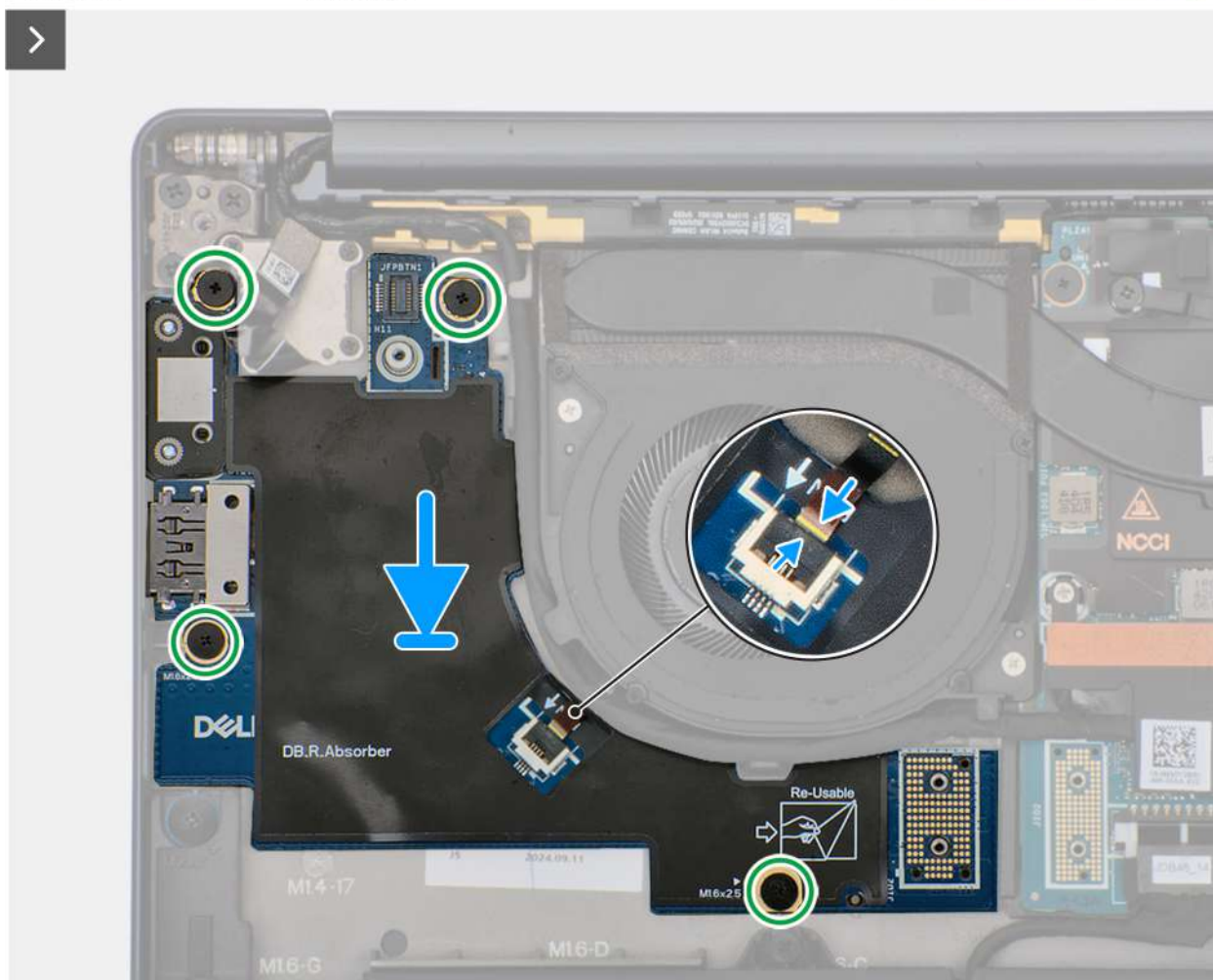
Figure 45. Installing the right I/O-board (without WWAN antennas)
