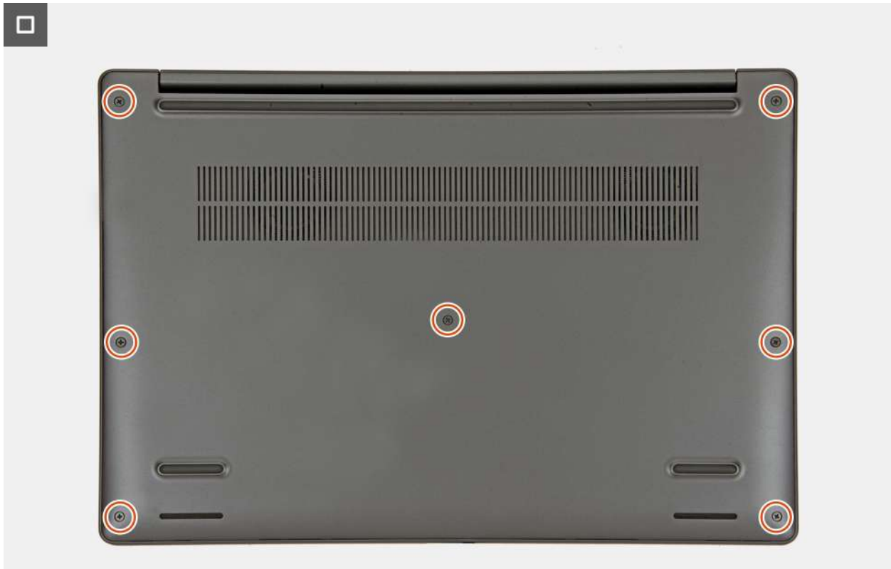
Figure 19. Tighten the captive screws
