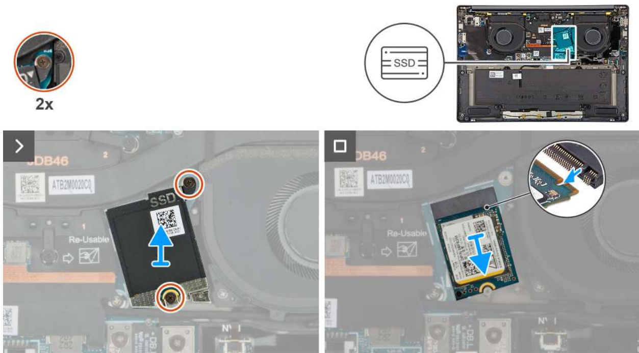
Figure 23. Removing the SSD
