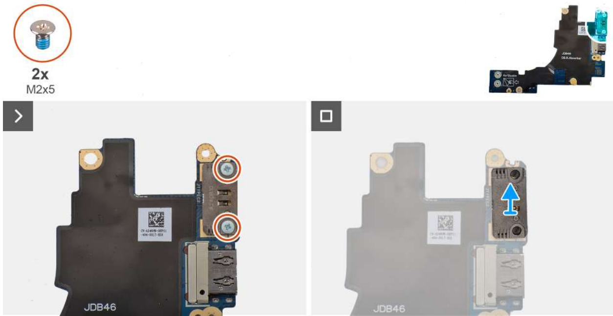
Figure 53. Removing the left USB Type-C module
