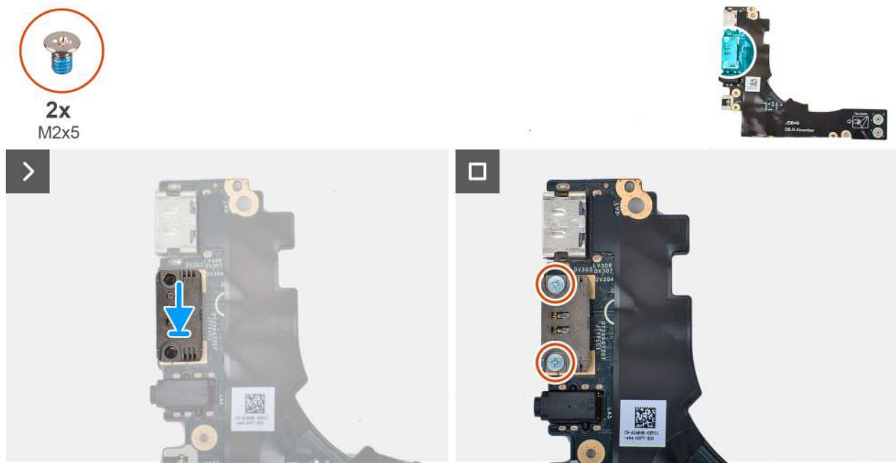
Figure 56. Installing the right USB Type-C module
