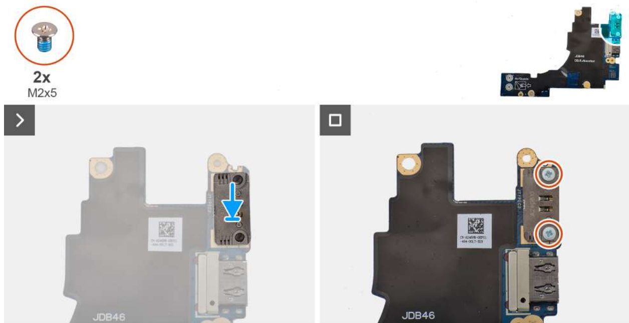
Figure 54. Installing the left USB Type-C module
