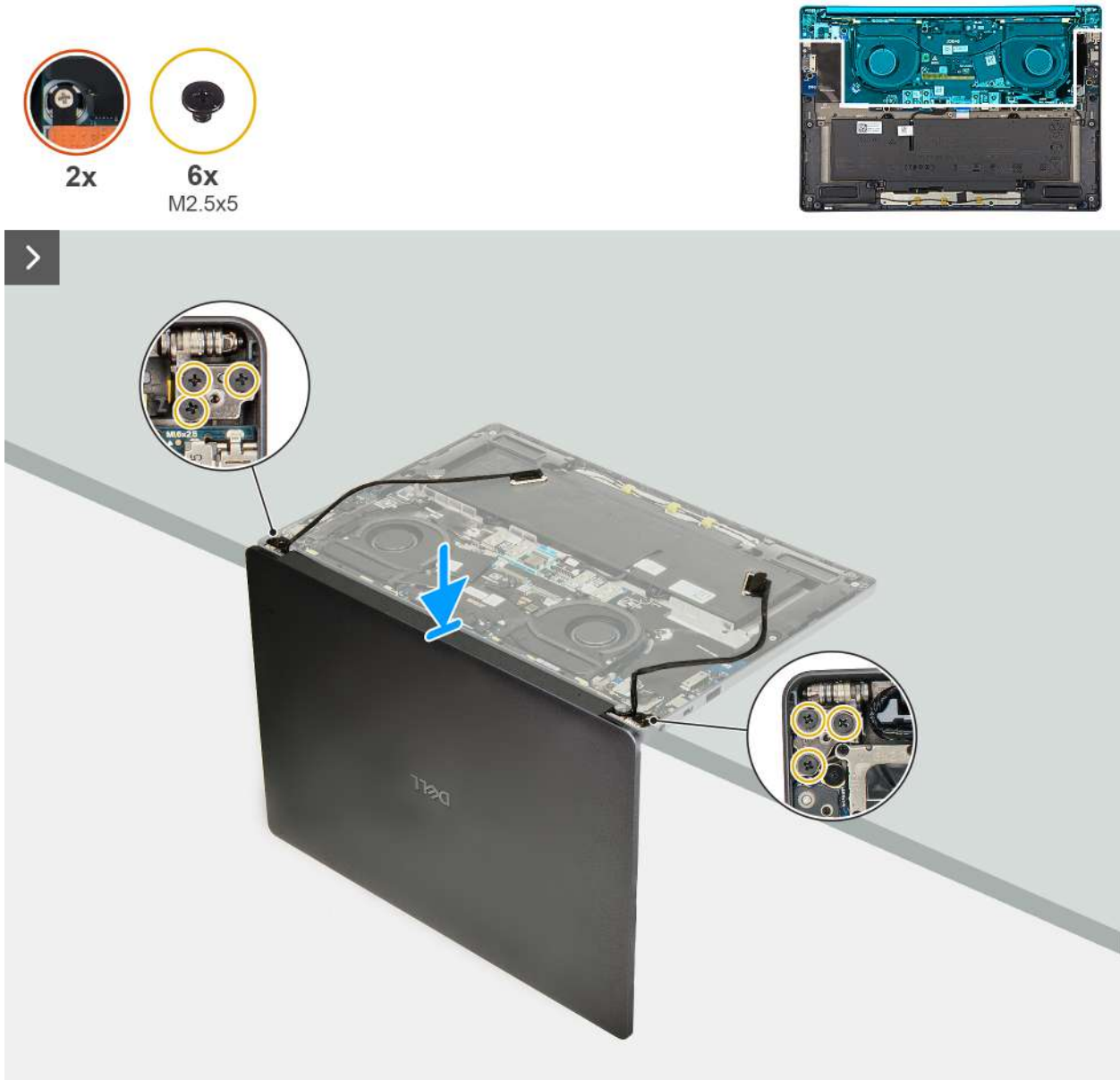
Figure 62. Installing the display assembly
