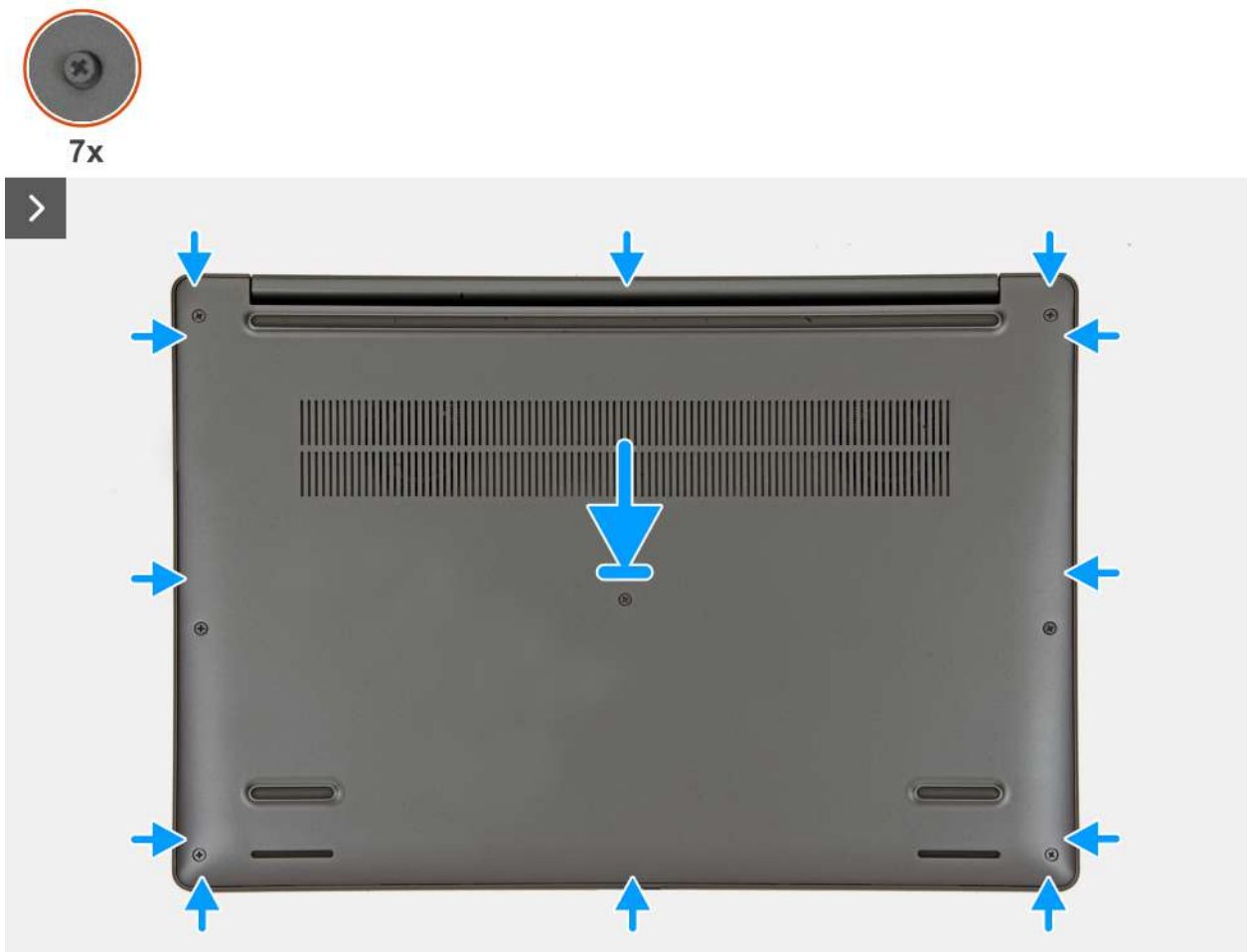
Figure 18. Installing the base cover
